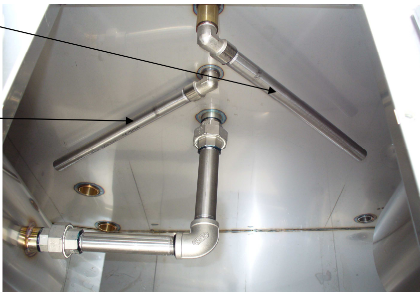
Water level maintenance solenoid valve pipe connection
