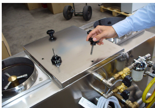
Unscrew the 4 fastening knobs to open the inspection door
